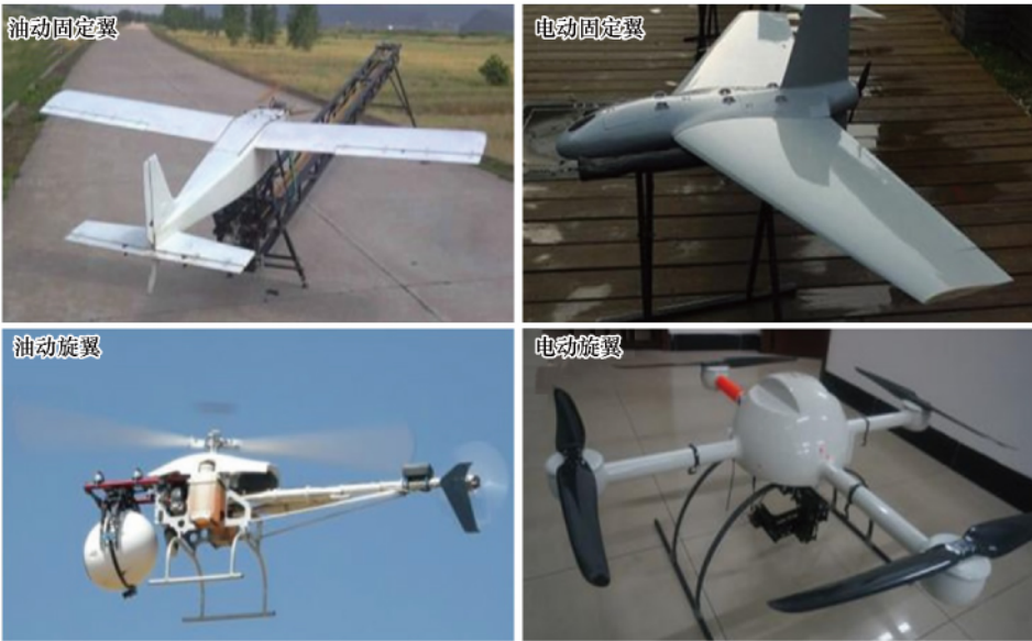
图 1 4 种主要民用无人机类型 Fig.1 Four main types of civilian drones
